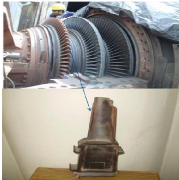
Fig 2: Position of First Stage gas turbine Blade on Rotor
